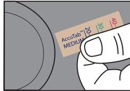
**3) Attach an ACCUTAB at the end of each strap.**
